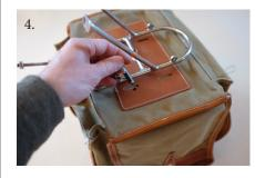
4. Make 5mm holes where you have made your marks. This can be done with a hole punch or nail. Use a wooden block or other means to support the bag from inside.
