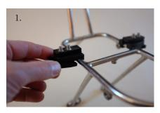
1. With the bag removed from the rack, postition assembled clips on rack in a clear and unobstructed postion, favoring a forward placement where possible.
