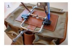
3. Disassemble the clips, leaving the retention bracket (D) in place. Mark the four holes on bag with marker or pointy tool.
